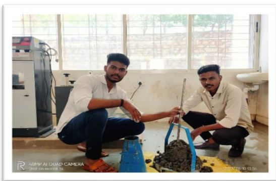
Fig. No. 1 Workability Slump cone test
