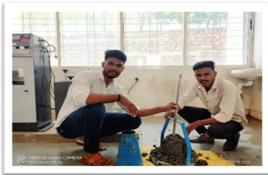
Fig. No. 3 Workability Slump cone test
