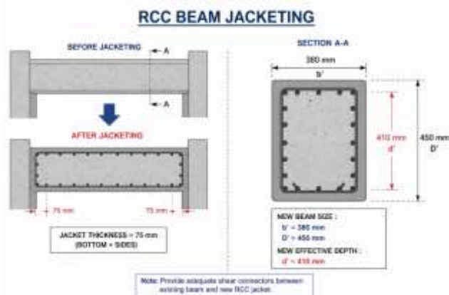
Fig. 5: RCC Beam Jacketing Detail
