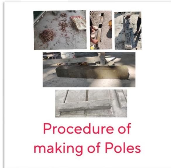
Image shows the procedure of making the poles using coconut shells.
