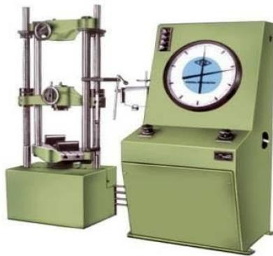
Fig.5.1 UNIVERSAL TESTING MACHINE
