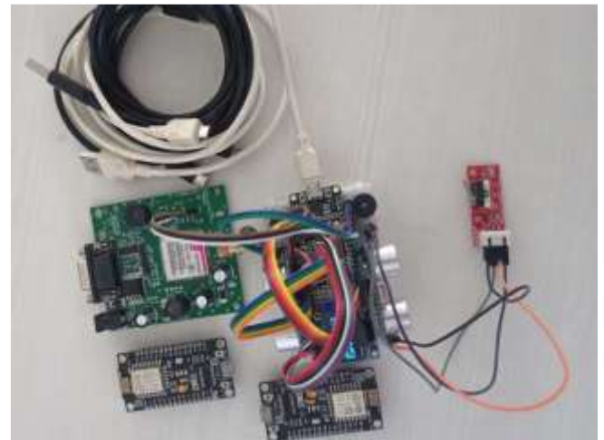
Fig 7.2: Impact/Tilt Testing of Accident Detection System
