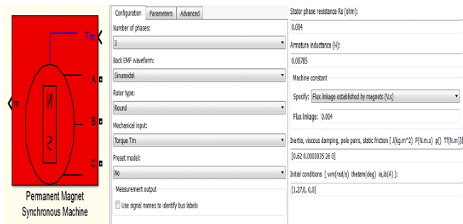
Figure 5.2: MATLAB Simulink block parameters for Permanent Magnet Synchronous Generator (PMSG).
