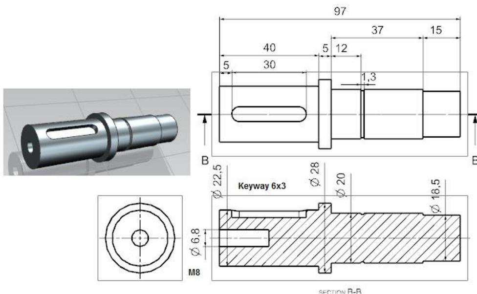
The motor shaft is designed for torsion failure:
