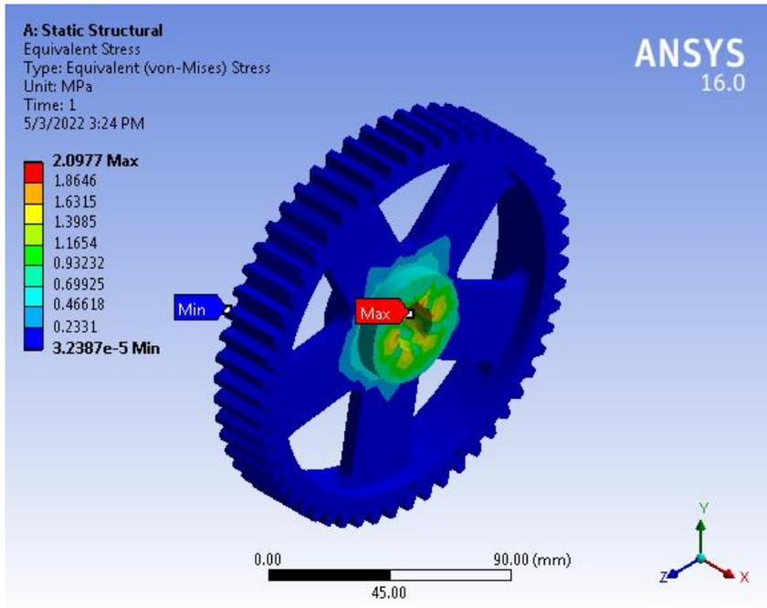
The maximum analytical stress is 2.89 Mpa which is far below the permissible limit hence the gear is safe.
