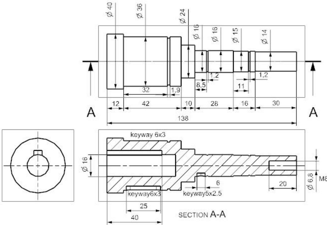
The motor shaft is designed for torsion failure:
