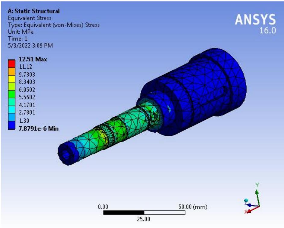
Maximum stress induced in the motor shaft is well below the permissible limit hence it is safe
