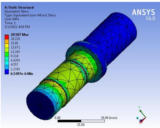
Maximum stress induced in the crank shaft is well below the permissible limit hence it is safe
