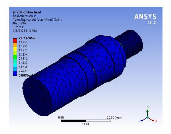
Maximum stress induced in the drill machine shaft is well below the permissible limit hence it is safe
