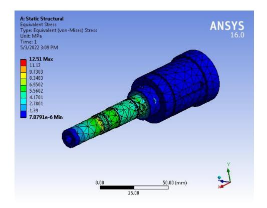
Maximum stress induced in the motor shaft is well below the permissible limit hence it is safe
