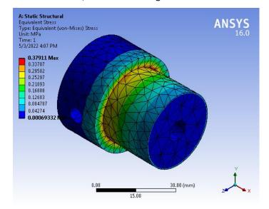
Maximum stress induced in the grinding wheel shaft is well below the permissible limit hence it is safe
