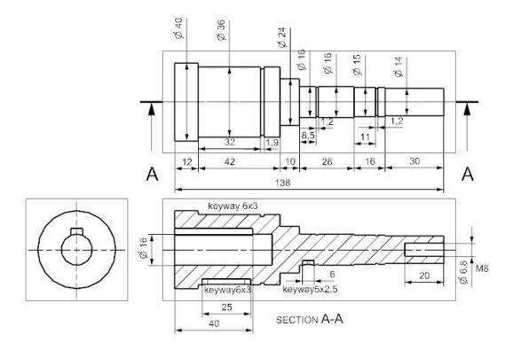
The motor shaft is designed for torsion failure:
