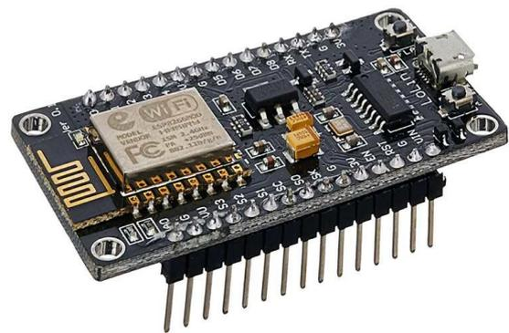
Fig -3: ESP8266 NodeMCU Controller
