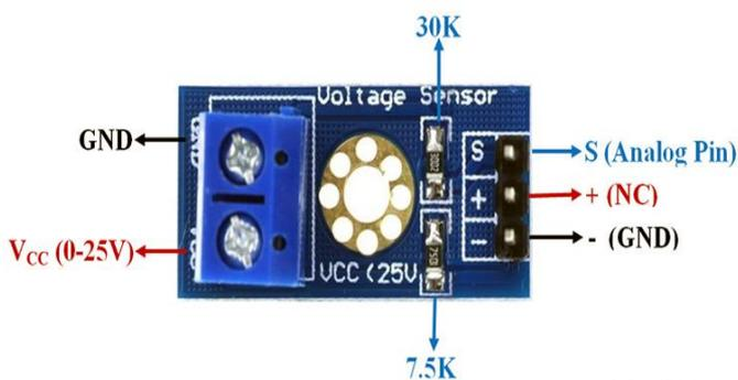
**Fig -6: Voltage Sensor**
