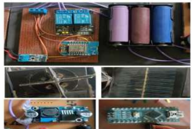
A1: Complete Hardware Setup of Solar Tracking System with Solar Panel, LDR Sensors, Servo Mechanism, Battery Module, Relay Circuit, and Microcontroller
