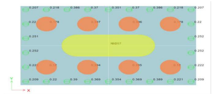
Fig 3.2 Punching Check b/w Pile & Pile Cap
