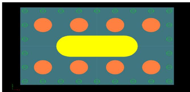
Fig 2 Plan View of Micro Pile & Pile Cap
