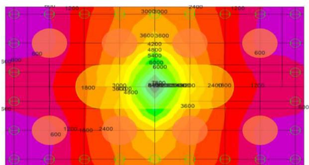
Fig 3.3 Maximum Resultant Bending Stress.
