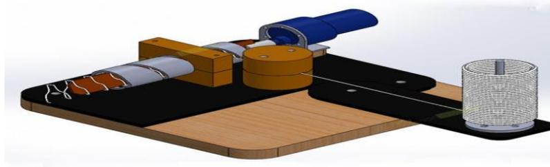
**Figure.1.8** Chain Link Wire Mesh Making Machine
