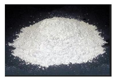
The inclusion of GGBS in geopolymer concrete requires careful consideration of its proportion in the mixture, as it can affect the setting time, workability, and mechanical properties. Researchers and practitioners have conducted numerous studies to optimize the GGBS content in geopolymer concrete to achieve the desired performance.
