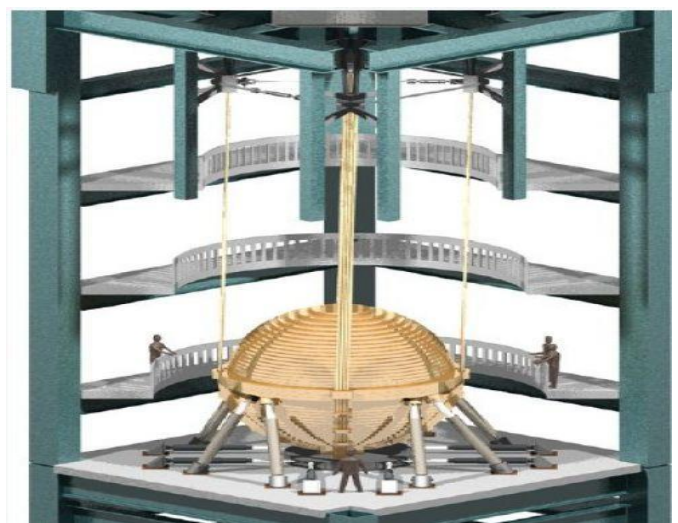
Fig -1: Tuned mass damper
