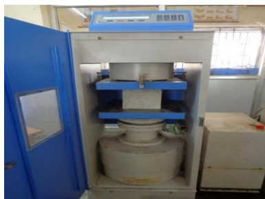
Fig -2: Compressive Strength Testing
