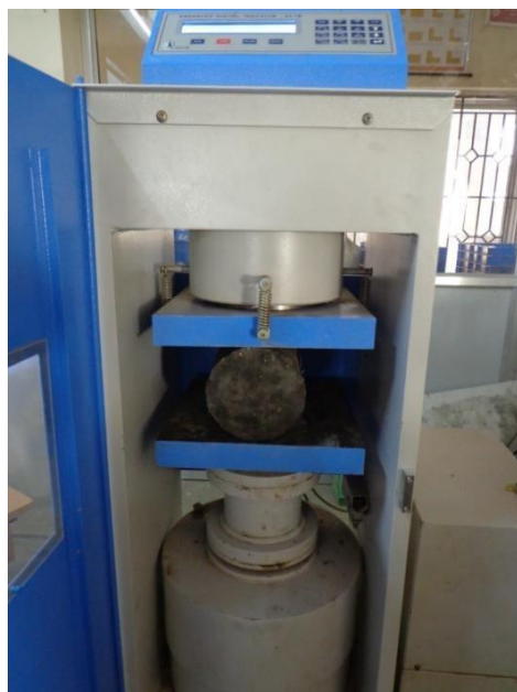
Fig -3: Split tensile Strength Testing
