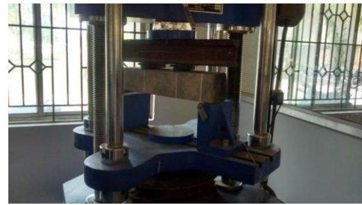
Fig -4: Flexural Strength Testing
