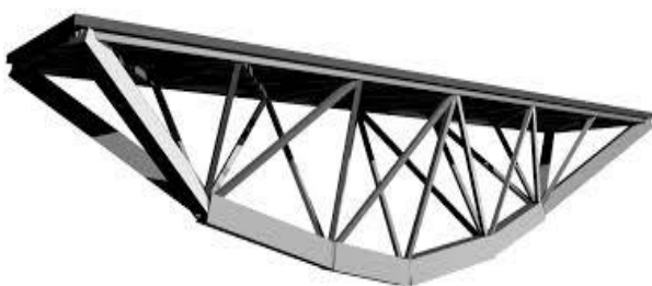
Fig. Truss structure with optimization
