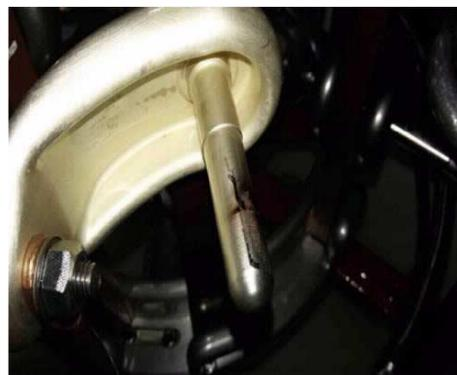
**Fig. 1 Arc traces at OLTC tap selector**
