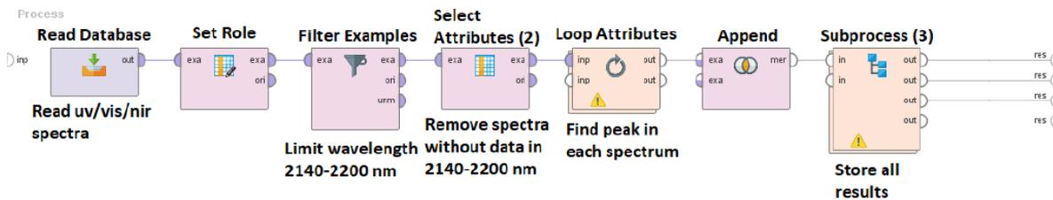
**Fig. 2 Algorithm for extracting spectrum files and storing in database.**
