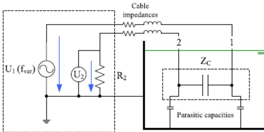
Fig. 3 FRA device connected to capacitive sensor.
