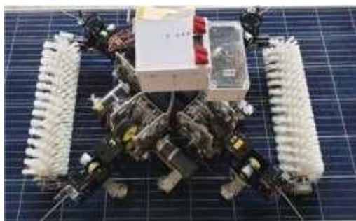
Fig.3.6.1-Four-side Stretch sling based solar cleaning robot [2]
