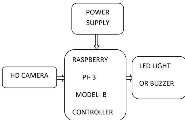
Fig3: Block diagram of Face mask detection system
