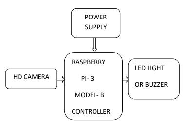
Fig3: Block diagram of Face mask detection system
