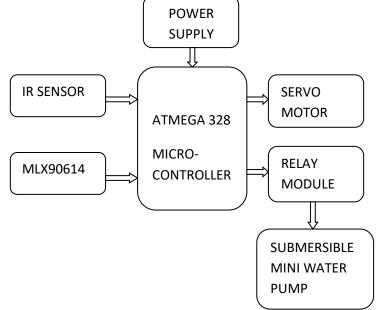
Fig4: Block diagram of Temperature, Sanitizer & Barrier System
