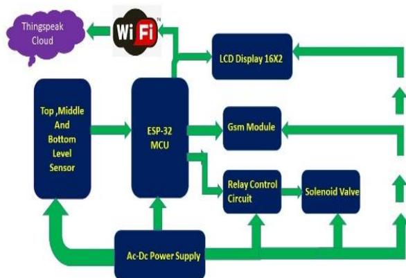
**Fig.1: IoT-Driven Infusion Monitoring & Management System**
