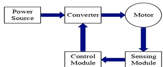
**Fig. 1.2Block Diagram of an Electrical Drive**
