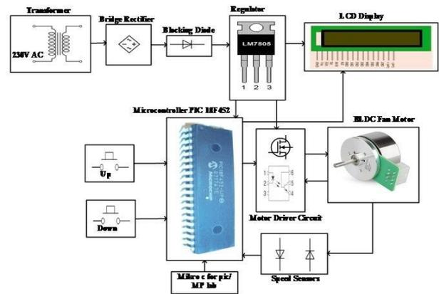
Fig. 6.1 Block Diagram
