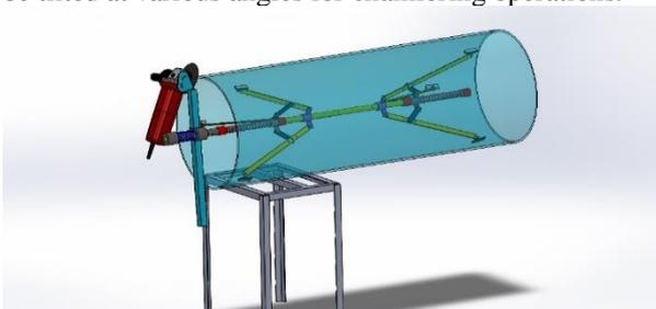
Pipe Chamfering Schematic cad dia.
