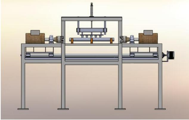
The conceptual design of double head chamfer machine is prepared or designed in Solidworks software and analysis in Ansys software. This project can conclude that the operations performing on this machine will overcome the disadvantage of conventional machine and will provide high-rate manufacturing with less time consumption and less consumption of manpower.
