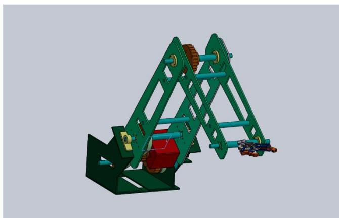
Fig 1: Proposed Robotic Arm
