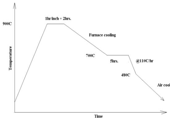
**Fig 1: Annealing heat treatment**
