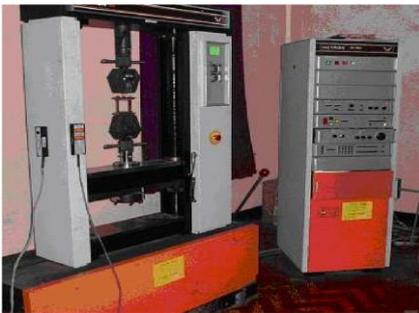
**Fig-2 Tensile Testing Machine**
