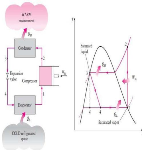
a low- quality saturated mixture. In evaporator, the refrigerant absorbs heat from conditioned space and completely evaporates. Leaving the evaporator, the refrigerant vapor re- enters the compressor at state 1 and finish the cycle.
