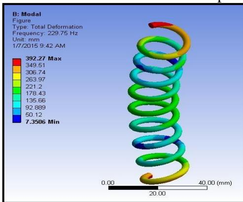
**Fig 1: Mode shape (7) and its Deformation**
