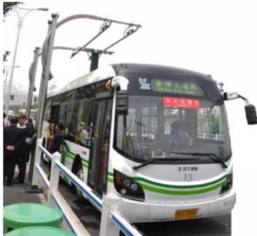
*It is a new form of electric bus powered via Energy stored in large on board super Capacitor. A connector in the roof connects to the stationary electrical installation when the bus stop to let the passenger on to the bus.*
