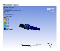
The maximum stress induced is 40.123  $\underline{\rm Mpa}$  is less than permissible stress hence the part is safe
