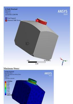
The maximum stress induced is 40.123  $\underline{\mathrm{Mpa}}$  is less than permissible stress hence the part is safe
