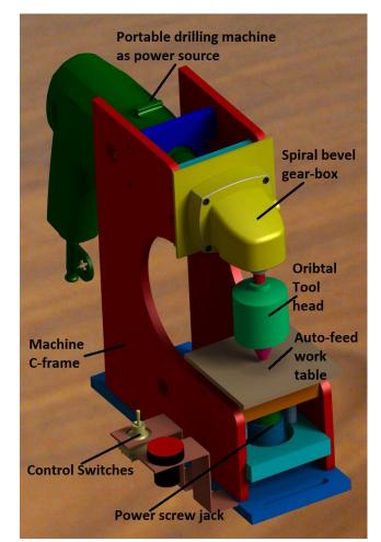
FEATURES OF OROPOSED ORBITAL RIVETTING MACHINE
