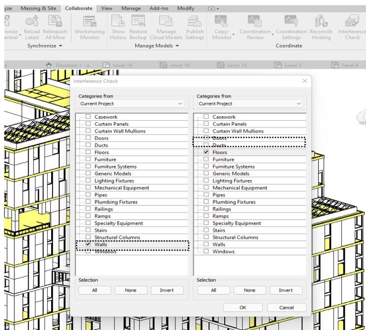
Fig(d) showing the Interference check Tab
