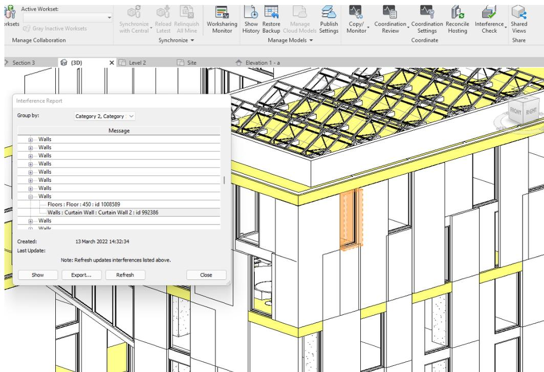
Fig(f) showing the Curtain wall that is clashing with the Floor above in 3d
