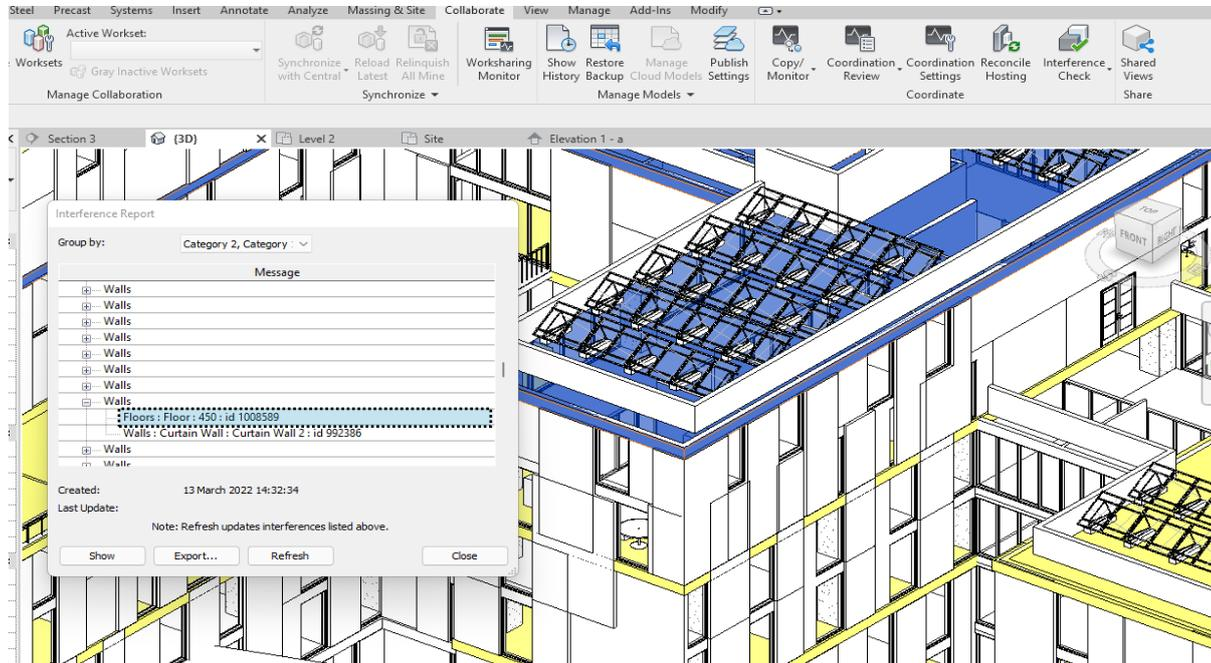
Fig(e) showing the Floor that is clashing in 3d
