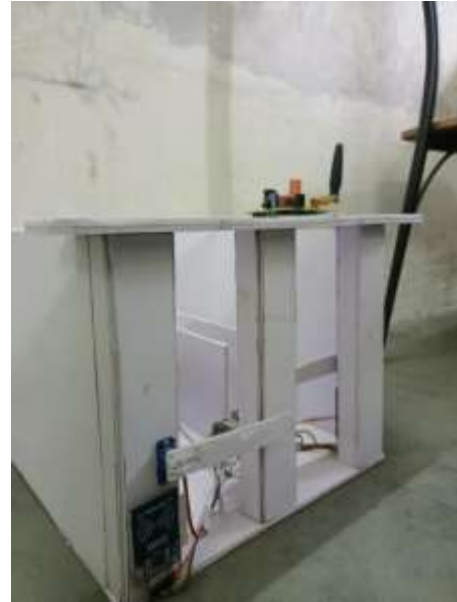
Fig. 5. Hardware Prototype — Side View showing RFID Reader and Gate Arm
