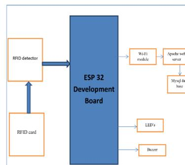
Figure 3.2 : Connection between the esp32 and other components.
