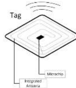
Figure 5. Functional Illustration of RFID Tag,
