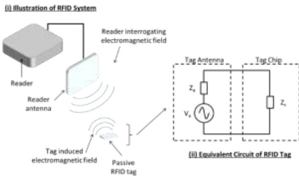
Figure 7. Principle of RFID Mechanism
