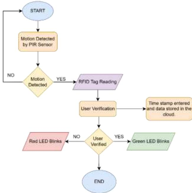
Figure 9. Algorithm of the RFID Attendance Monitoring System.
