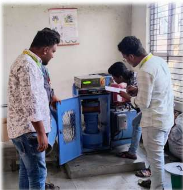
Fig -5: Compressive strength testing of brick specimen using a compression testing machine
