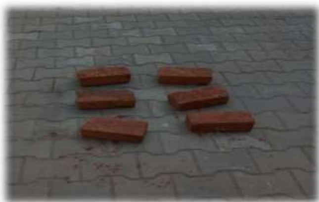
Fig -4: Manufactured brick specimen prepared from red soil, fly ash, gypsum, lime powder and coconut shell powder
