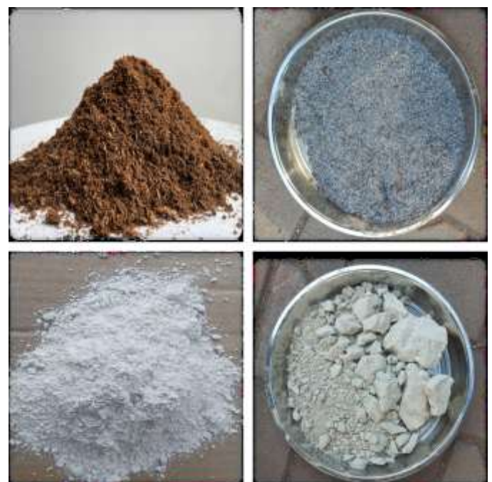
Fig -2: Raw materials used in brick manufacturing — (a) coconut shell powder, (b) fly ash, (c) lime powder, (d) gypsum
