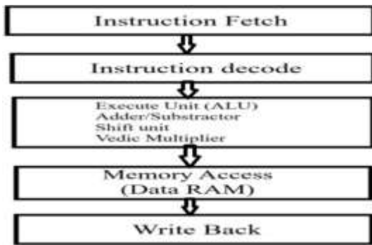
Fig.1: Flow diagram of 5 stage pipelined RISC-V Processor with integrated 2bit Vedic multiplier
