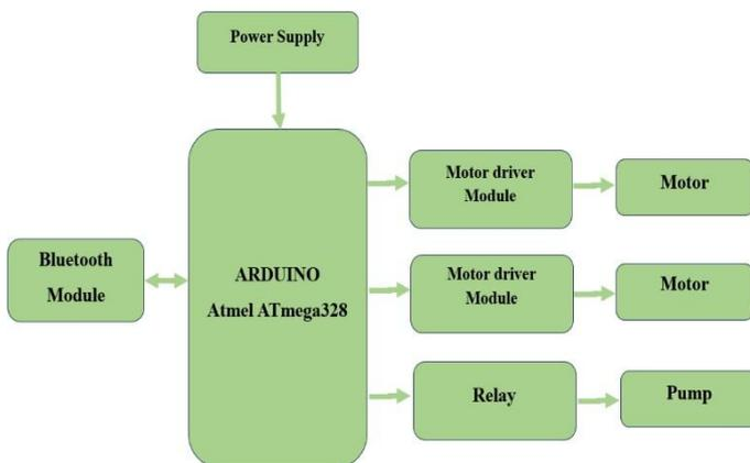
The block diagram illustrates a robotic pesticide spraying system based on an Arduino Atmel ATmega328 microcontroller. The system is powered by a power supply that provides the necessary voltage to the Arduino and other connected components. A Bluetooth module is integrated with the Arduino to enable wireless communication, allowing remote
