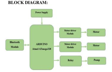
The block diagram illustrates a robotic pesticide spraying system based on an Arduino Atmel ATmega328 microcontroller. The system is powered by a power supply that provides the necessary voltage to the Arduino and other connected components. A Bluetooth module is integrated with the Arduino to enable wireless communication, allowing remote control of the spraying mechanism.
