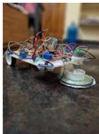
Fig -11: Robot prototype for cleaning solar panel
