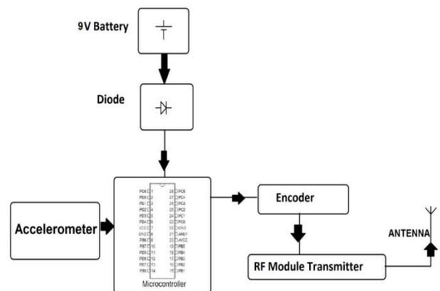
**Figure1. Circuit Diagram of Transmitter**
