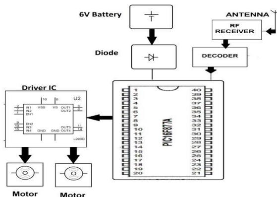
Figure2. Circuit Diagram of Receiver
