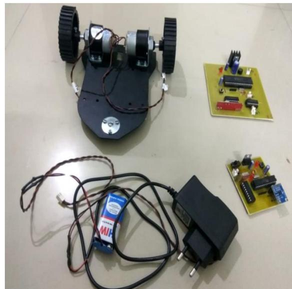
**Figure9. Unassembled image of robotic vehicle**
