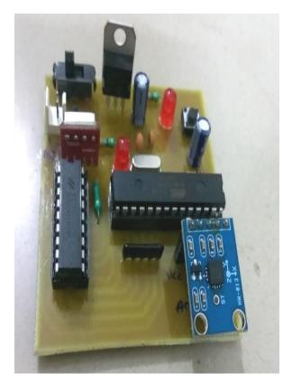
Figure4. Circuit image of Transmitter
