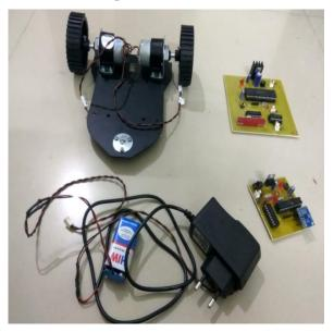
Figure9. Unassembled image of robotic vehicle
