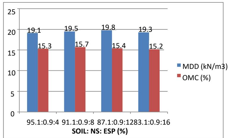
Fig.4.2.2: Graphs representing the MDD and OMC value of various mixes together.
