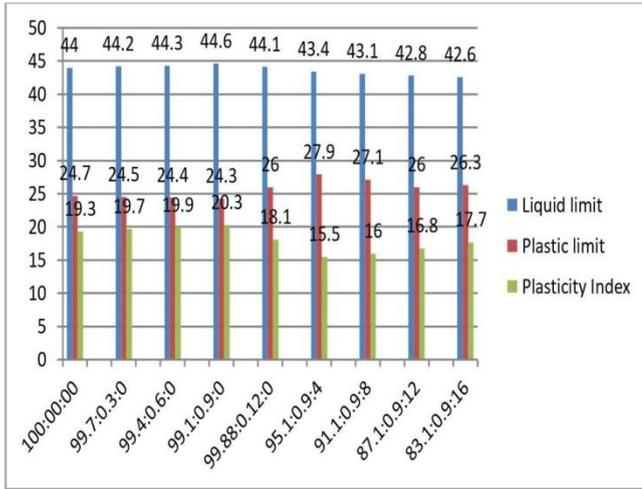
4.1.1 Graphs representing the Liquid limit, Plastic limit and Plasticity index value of various mixes.
