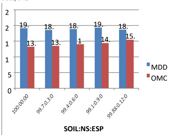
Fig-4.2.2 Graph representing the MDD and OMC value of Soil: NS
