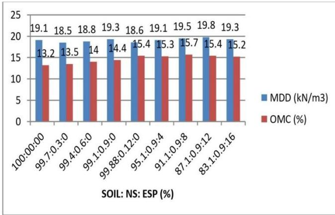
FIG. 1.2: Graphs representing the MDD and OMC value of various mixes together
