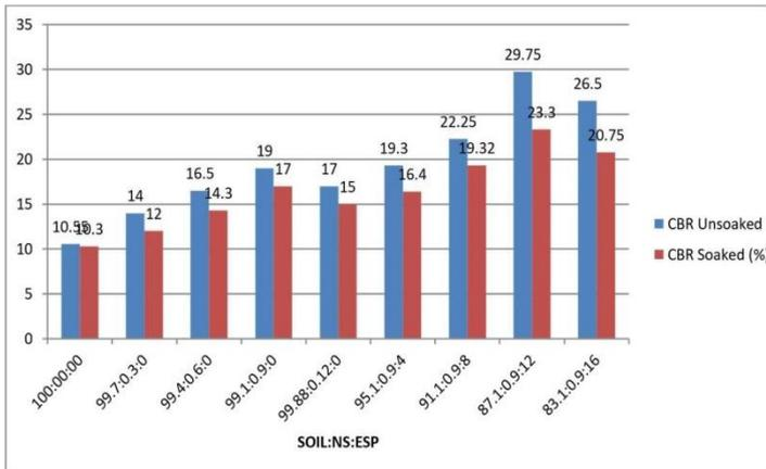
**FIG.4.4.1: GRAPHS REPRESENTING THE CURVE THAT ARE OBTAINED FROM CBR TEST FROM SOIL NS ESP MIXTURE.**
