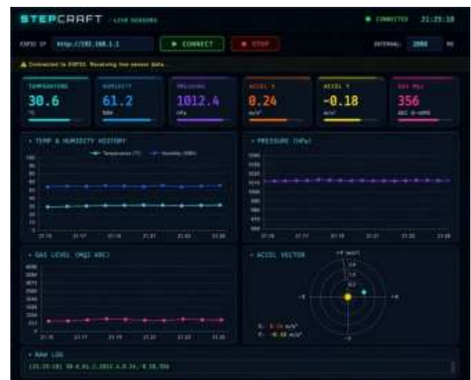
Fig4: Real-Time Web Dashboard for RTOS-Based Satellite Telemetry Monitoring System
