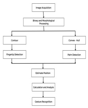
Fig.6: Workflow for Hand Detection
