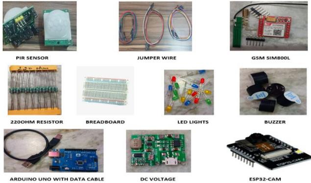
Fig.5: Devices Used in the System
