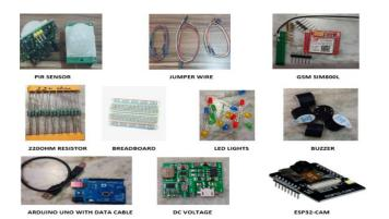
Fig.5: Devices Used in the System
