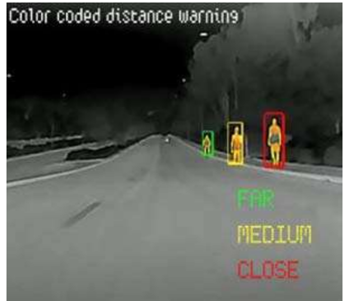
Fig. 7. Human Detection in Night Vision Mode
