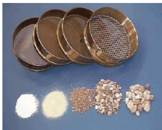
. Fig: sieve Analysis Of Quarry Aggregate
