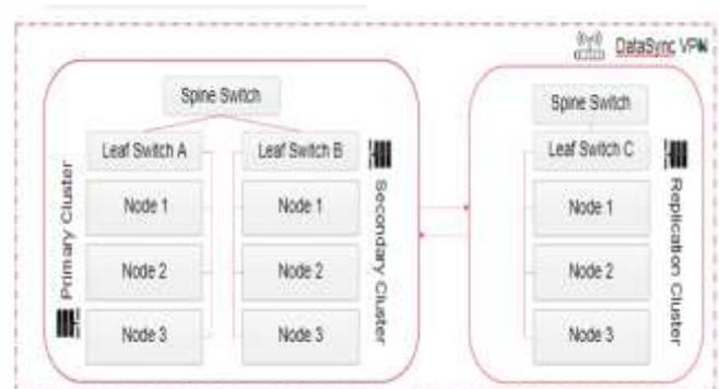
Figure 2 DataSync Hub - Clustering Architecture
