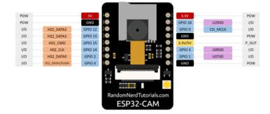
Together with a camera module, the ESP32-CAM is a potent microcontroller that has built-in Bluetooth and Wi-Fi. Its main duties in the drone are people detection and image capturing. The module has an integrated camera that can record video and take pictures; this is usually an OV2640.
